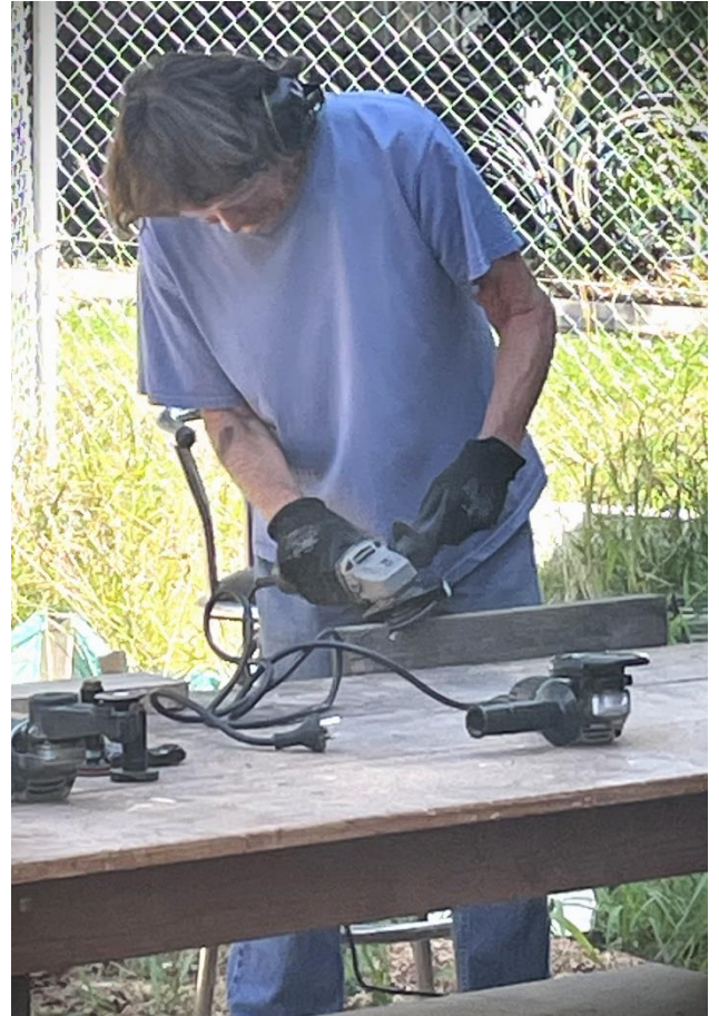
Demonstrating how to hold the tool and his stance. Protective gear in the form of gloves, earplug and goggles were essential.
