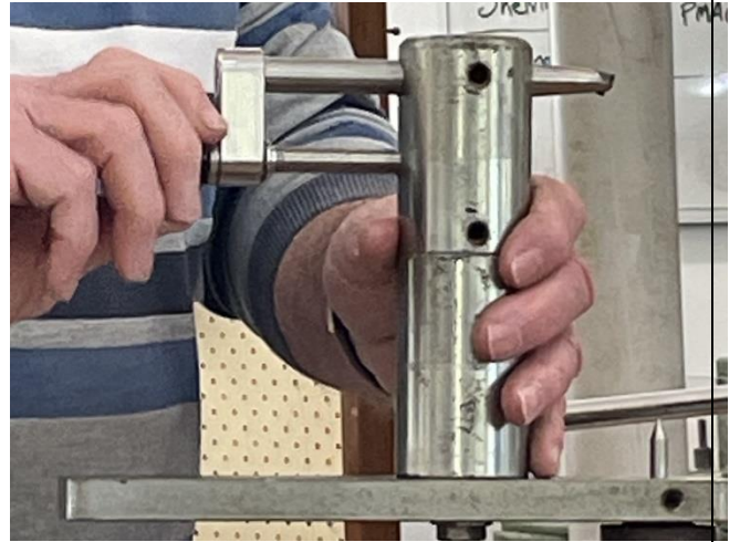
Set on lathe bed, then moved in a curve to create the sphere.
