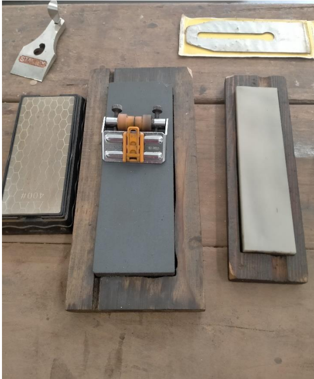
Special attachment to set the angle of the blade whilst being sharpened.
