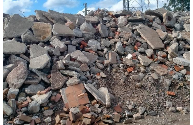
Image 2 shows the area for dumping concrete waste which is ground up into gravel, 40mm and 80 mm, to be sold off.
