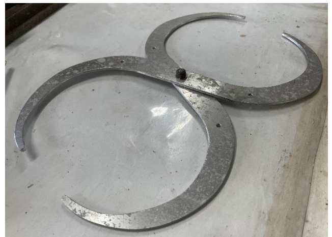
Callipers made from aluminium. Used to measure the thickness of the walls of a bowl.
