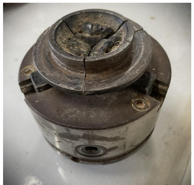
The jaws of this chuck can be removed and realigned. This enables off-set work the be set-up.
