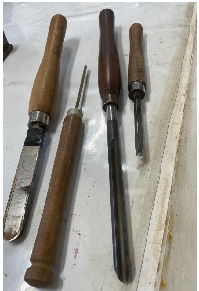
David enjoys lathe work. Many of his chisel are made by him. In the above, the 3 rd one from the left is a bought one. The one on the left is heavy gauge with toughened steel cutting edge.
