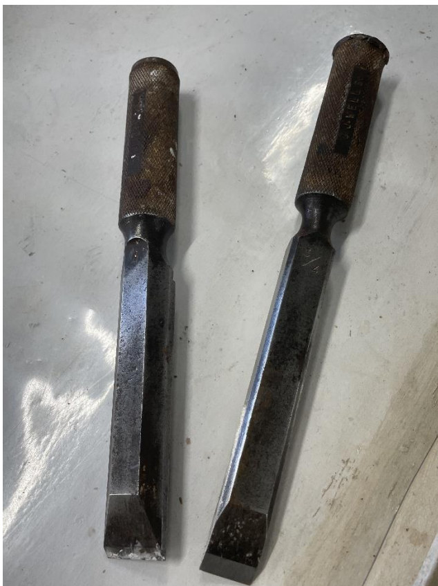
Solid wood chisels. David has always been told to never hit a wood chisel with a metal hammer – too
