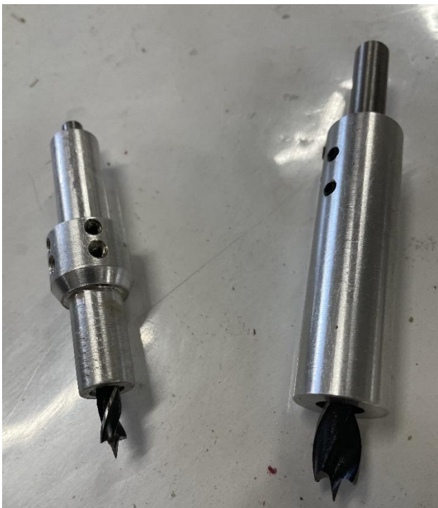
Casings for brad bits to keep them on task. The plug hole and thread were done by David.
