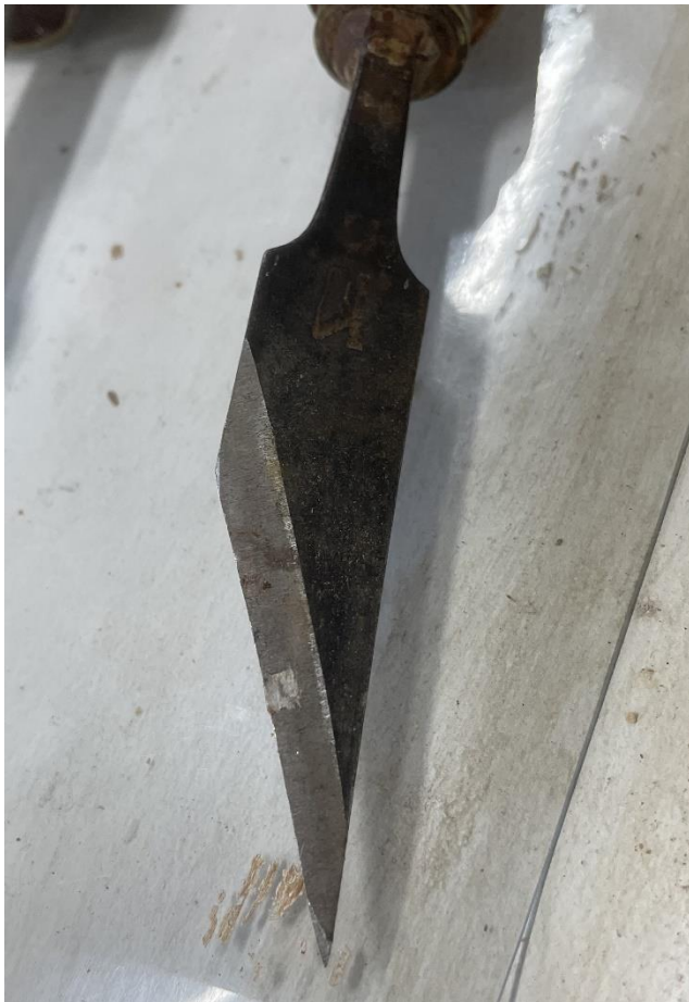
When using a lathe, a skew chisel is useful. However, David wanted a chisel with a longer blade so he made it.
