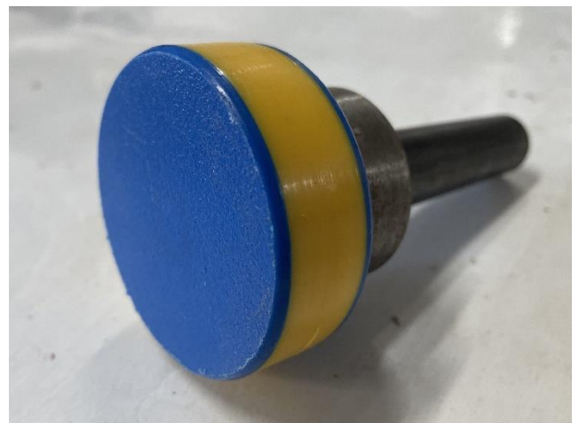
Used on the lathe at the dead stop. Good for pressing a job against it so it doesn't wobble and fall off. Especially helpful with off-set work.
