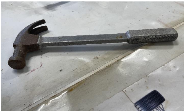
He needed a hammer, but the handle was broken. Made a steel handle with grip.
