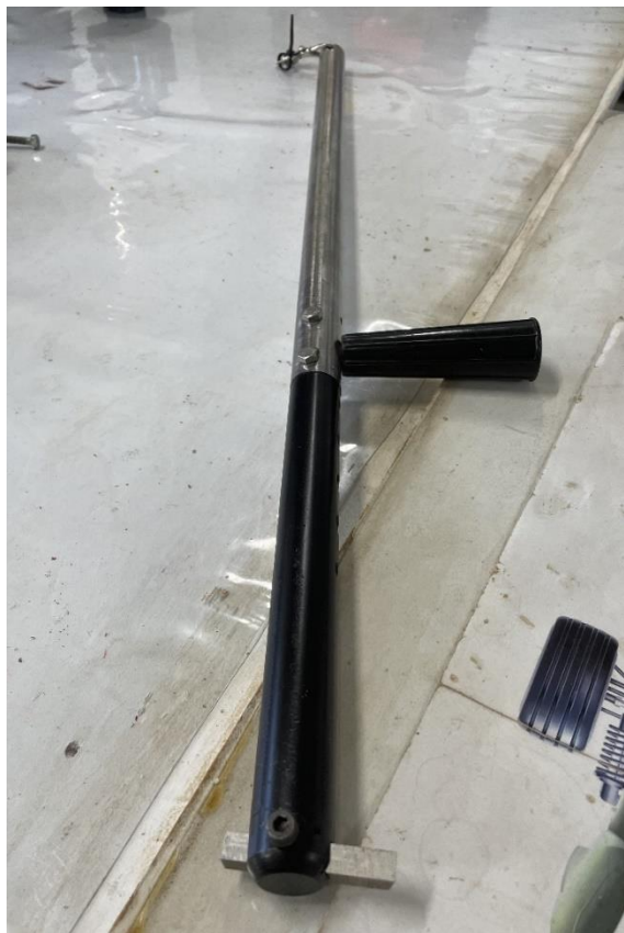
Named "The Beast". Used to clean out the insides of large bowls. Cutting edge at the bottom of image.
